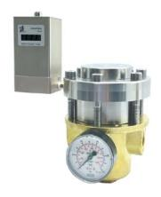
This Proportional Pressure Regulator provides pilot pressure to the ratio relay volume booster. By controlling pilot pressure at the top of the diaphragm, we can control the output pressure of volume booster. Volume booster is also called a dome-loaded or pilot-operated pressure regulating valve, which can be used as pressure regulating valve or back pressure valve.
